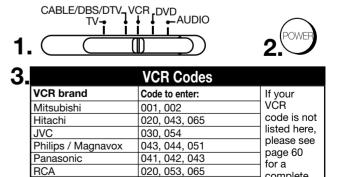
To reset to default code, enter 000 Figure 3. Programming the remote to control your
